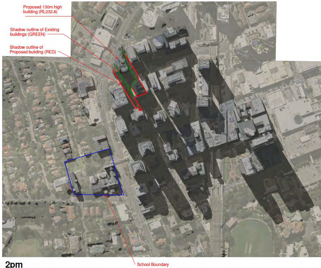
Figure 39: Solar study 2pm (Source: Solar Study, FJMT)
